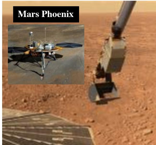
Autonomous digging: Digging while modifying digging behavior based on sensed hardness of Martian soil.
