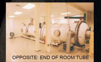
3 by12-m test volume for baffle or mirror 1.3-m diameter, 82-m long section 1.5-m diameter, 10-m isolatable section Pumped with cryo-pump: <10<sup>-7</sup> torr Measured baffle rejection ratios up to 10<sup>15</sup> Use to test x-ray optics up to 1-m dia
