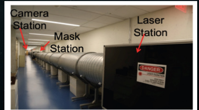
Starshade test bed at Princeton University.
