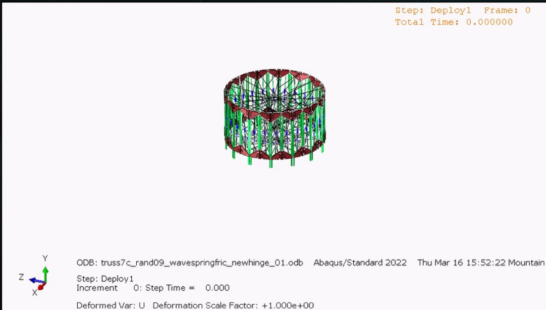
Deployment model of inner disk testbed built for previous milestone
