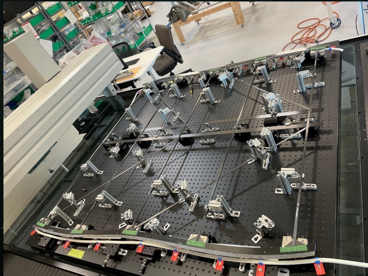
6 m-long petal section being assembled
