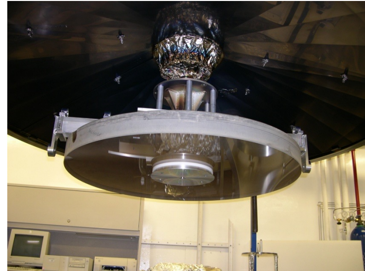
Mirror mounted in 2-meter chamber prior to coating
